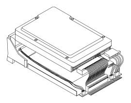
8. Secure the drive to the tray with four screws.
